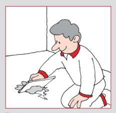
The substrate should be cement / concrete based and holes and weak parts should be repaired with frost proof and waterproof cement mortar.
