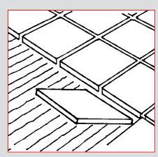
20-30 hours after application the surface is ready for tiling.
