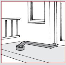
Wall to floor joints and joints in concrete should be sealed with the safecoat roll, except on cast reinforced concrete like swimming pools, water reservoirs and the like.
