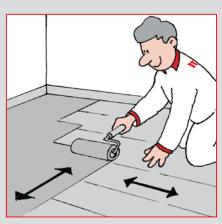
When application is touch dry on walls and safe to walk on floors apply second layer with same amount to a total of 2.2 - 2.5 kg/  $m^2$ .
