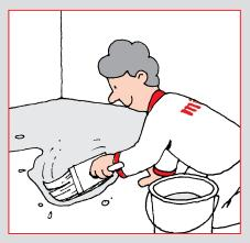
Dry and absorbent substrates should be moistened with water or primed with diluted 4180 primer.
