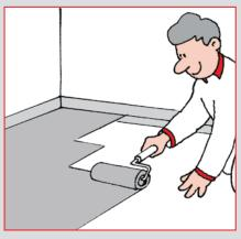
The whole area should be coated with 4650 aquastop flexible using a brush or roller.
