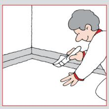
Cover the safecoat roll with 4650 aquastop flexible.
