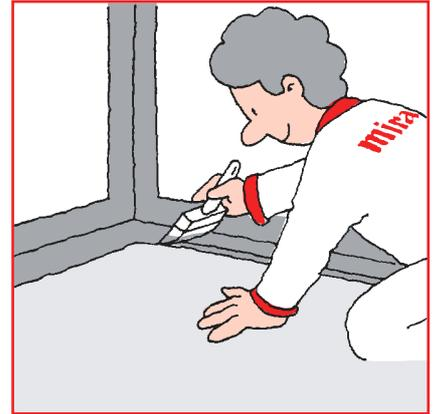
Cover the safecoat strip with a further coat of 4400 multicoat, ensuring that it is fully covered. The 4400 multicoat should extend 100 mm up the wall.
