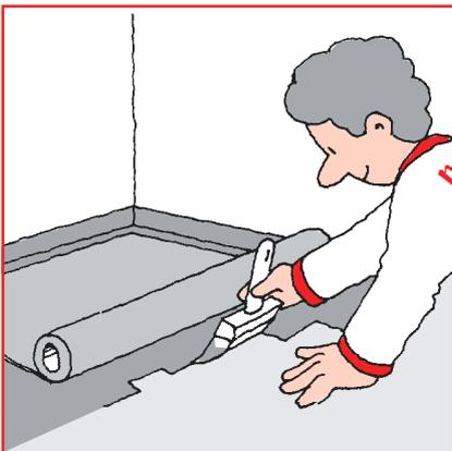
Start to coat the floor with 4400 multicoat and simultaneously cover with safecoat, rolling the material into the coating.
