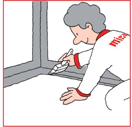
The safecoat strips should be covered with another coat of 4400 multicoat, ensuring that it is fully covered and absorbed. The 4400 multicoat should extend 100 mm up the wall.
