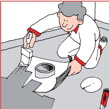
Around pipes the appropriate safecoat manchete should be used. Cut a hole in the "manchet" slightly smaller than the diameter of the pipe, place the "manchet" over the pipe and press down firmly against the floor. After fitting saturate the "manchet" with 4400 multicoat.
