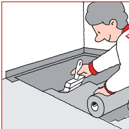
A second coat of 4400 multicoat should be immediately applied to the safecoat making sure that the material is fully covered and saturated. To check for complete waterproofing of the surface ensure that no traces of the original white colour of the safecoat remain.
