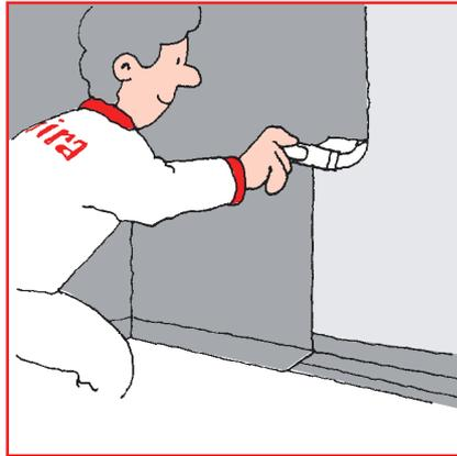
In the "wet-zone" (see diagram on back page) a min of 1 mm (1,25kg/m<sup>2</sup>) 4400 multicoat should be applied. If applying more than one coat, the first should be dry before the next is applied.
